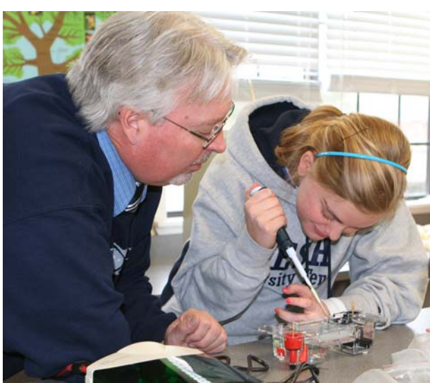
Dr. Baker's AP Biology students are using equipment on loan from LSU to isolate and study their own DNA. They have taken DNA from their own cheeks and amplified it (DNA amplification using Polymerase Chain Reaction). Using pipets, the students are injecting the DNA into gel, which they are then putting through a process called DNA Electrophoresis, which sends an electric current through the gel, causing the DNA fragments to separate. They will examine the results to determine which samples have a certain gene that is fairly new in human evolution and only present in some individuals. In addition, to samples of e coli, they have added a glow-in-the-dark gene, which they will put on plates and examine.
